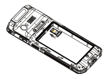
Step 1: Slide the battery cover latch to the unlock position and remove the cover and battery.
